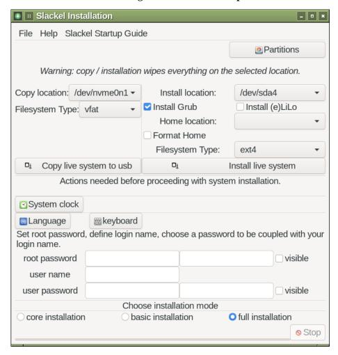
Then click on "Copy live system to usb" button to begin the installation on USB.
